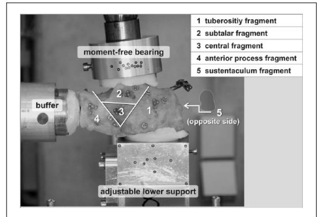
**Figure 4.** Fracture model and holding device mounted within the servohydraulic machine.
